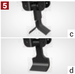
BLADE OPTIONS: a) Hammer blade: for heavy-duty operation. b) Straight blade: wheat, rye, barley, rice, etc.; c) Universal Y blade (optional): for all types of crop residue, e.g. maize, sunflower, sugar beet, cotton, grass, weeds, etc. d) Flail hammer blade.
