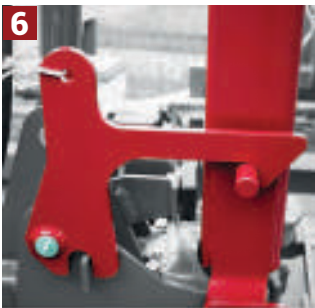
SECURING THE MACHINE in the transport position
