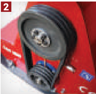
LATTERAL TRANSMISSION through toothed V-belts
