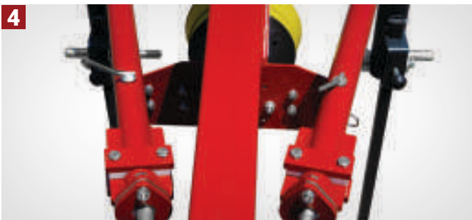
LATERAL SHOCK ABSORBERS By removing the shock absorber lock, it is possible to move the rake relative to the tractor direction by \pm 25^\circ , allowing the tractor to turn without lifting the machine and without stopping raking. They also have an important function in ground contour adaptation.
