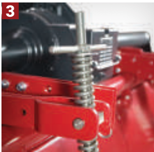
REAR HOOD position setting adjusts the level of soil pulverization
