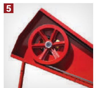
A SET OF V-BELTS transmits power to cutter bar driveline.
