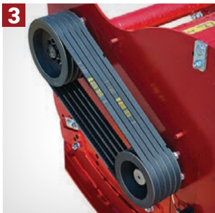
LATERAL TRANSMISSION through toothed V-belts.
