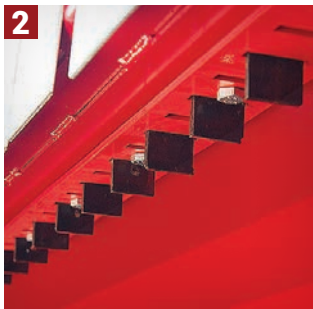
COUNTER BLADES enable better shredding of cover residue. One set is standard + option for fitting one more set (for straw etc.).
