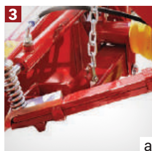
FRAME: a) Safety system for automatic release of the cutter bar in case of obstacle impact; b) Hydraulic lifting system (optional);
