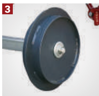
THE WORKING DEPTH is adjustable with a 2-wheel frame
