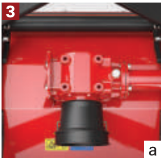
GEARBOX with overrunning clutch: a) Rear-mounting (standard); b) Only front or combination of front and rear mounting (optional).
