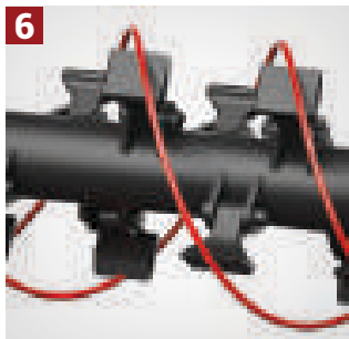
PRO SERIES with rotor 198mm diameter, electronically balanced with heavy forged hammer blades
