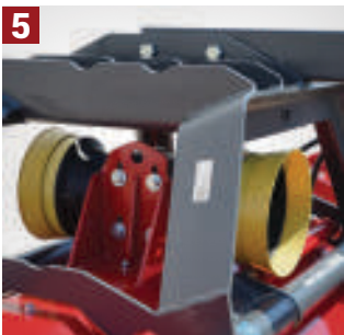
GEARBOX with two output shafts for front and rear attachment
