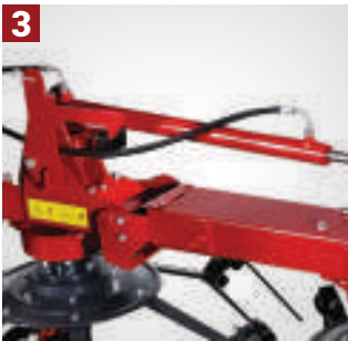
HYDRAULICS SYSTEM to move the machine from working to transport position
