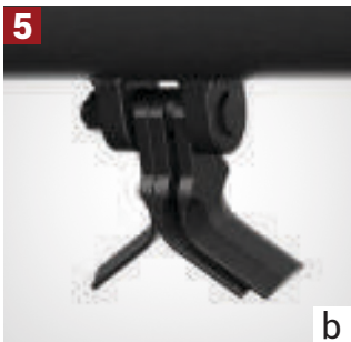
BLADE OPTIONS: a) Hammer blade (standard) - for difficult operating conditions (branches, thicker weeds, grass, etc.); b) Universal Y blade (optional) - for easy operating conditions (grass, weeds, etc.).
