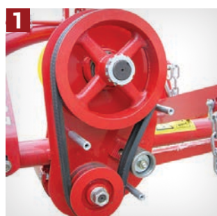
TRANSMISSION through V-belts with belt tensioners.
