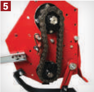
TRANSMISSION Chain drive transmission in oil bath
