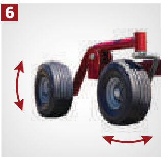
VERTIC. WHEEL MOVEMENT by \pm 10^\circ improves ground contour adaptation. Turning the first pair of wheels allows the tractor to change direction without lifting the machine.
