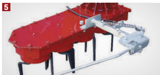
SIDE MOVEMENT is realized with the sensor spring
