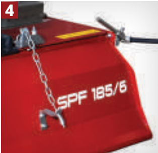
REAR HOOD position setting adjusts the level of soil pulverization
